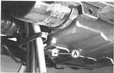
A. Engine Oil Drain Plug
